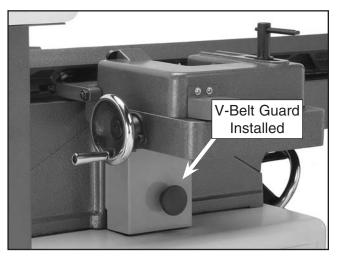
Figure 7. V-belt guard installed.
